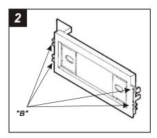
Cut and remove all mounting tabs on the *Radio Housing* EXCEPT tabs "B". The mounting tabs can be identified by the stamped letter on the back of each tab. *Skip to the Installation Instructions for ALL VEHICLES on Page #5.*
